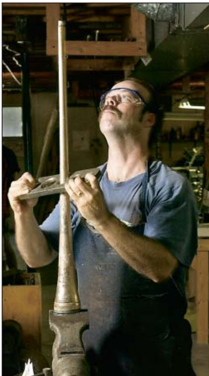
A HORN'S TAIL: Paul Lawson shapes the tail, the long piece that connects the end of the French horn with the rest of the tubing. He slides a metal mold over the tail to help give it a round, smooth surface.
