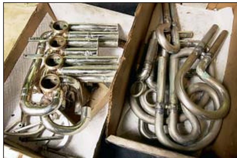
WAITING FOR ASSEMBLY: These French horn parts include four circular valves (l.) that control the air flow through the tubing (r.).
